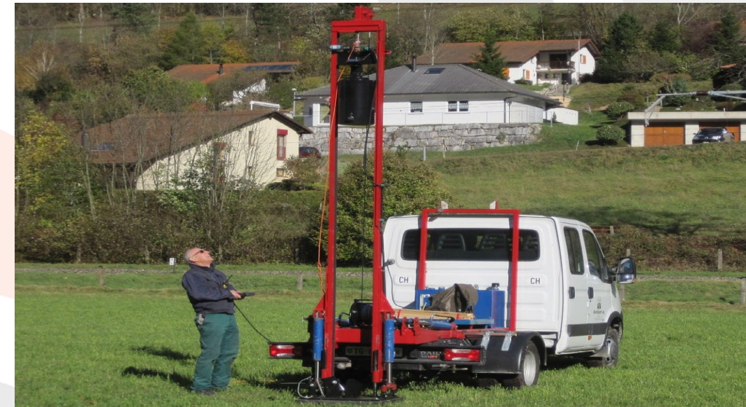
Free fall weight drop seismic source. Image sourced from GeoExpert AG
