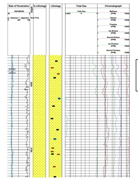
SF7u – Part of the mud log (live measurements from drilling ops) showing massive increase in Total Gas % and Methane Concentration exceeding 10,000 ppm in reservoir
